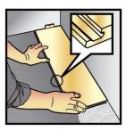
**Step 2.** The next board is installed at an angle (approx. 30°) against the end- joint and pressed down.
