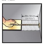
**Step 5.** Snap another chalk line from the first row at plank width. Trowel adhesive to chalk line. Start the second row with the off-cut from the first row, which must be a minimum length of 50 cm. Click this board to the previous row.
