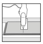
**Step 6** Min. length of the first plank is appr. 500 mm (20 in). Put a spacer toward the wall.
