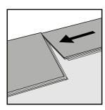
**Step 9** Fold the plank down in a single movement with a slight press to the eft to the short end of the previous plank. Ensure the planks are tight against each other both during and after this step.
