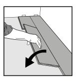
**Step 10** First row. Adjustment to an uneven starting wall. Copy the wall line to the first floor plank row iwth the shown tool, disassemble the 2 or 3 rows (see instruction below), adjust planks and reinstall.
